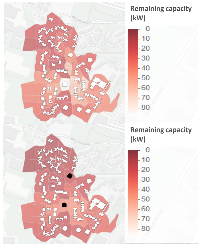
Fig 1: Cap'ten user interface, with initial then dynamic estimation (two new loads: black points)
